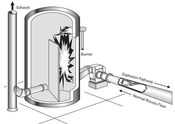
Figure 1: Unprotected Vapor Collection System
