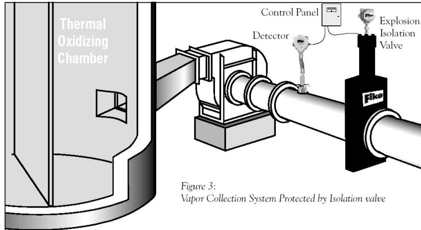
**Figure 3: Vapor Collection System Protected by Isolation Valve**
