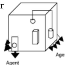
If the room's air-moving equipment is off during the retention period, the agent will drain out-much like water out of a hole in a bucket. Air will then flow in through the upper leaks.
