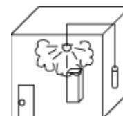
After discharge, the heavier-than-air agent pressing down upon the floor creates a small positive pressure. Flow develops whenever holes have pressure across them. The greater the pressure and the larger the hole, the greater the agent lost. As the agent runs out the bottom, a small negative pressure develops at the top. This pulls air in through the higher level leaks. Each agent creates a slightly different pressure as indicated by the densities as shown in the standards.
