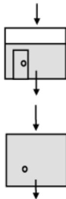
The intersection between the pool of agent below and clean air above is referred to as the agent/air interface. This is called the descending interface case. This interface drops, as agent is lost from the room through leaks in the floor and lower wall area. Air from outside the room replaces the lost agent by infiltrating through leaks in the upper half of the room.
